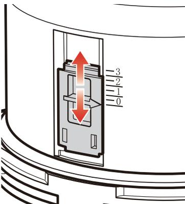
7. Adjust the full flush volume by sliding the red part up or down. when the buoy is higher, the discharge water volume is less. slide down the part can buoy little until you are flushing enough water.
