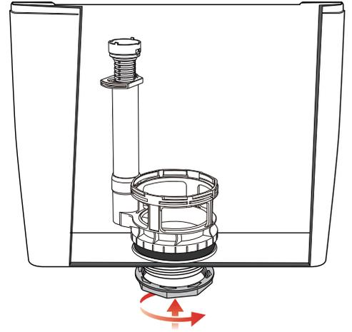
3. Insert the flush valve's base into the water tank. Screw on the hex nut properly.
