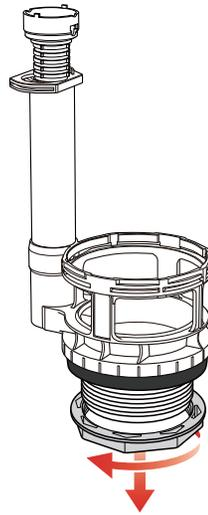
2. Remove the hex nut from flush valve base. Don't remove the seal !!!
