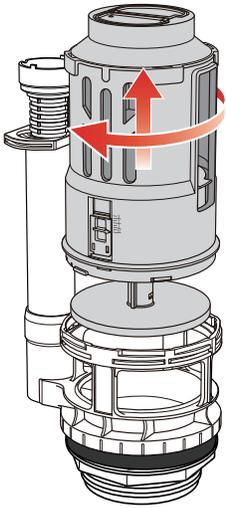
1. Hold the base of the flush valve and rotate the body counterclockwise. Take it out from base.
