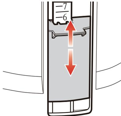
8. Adjust the half flush volume by sliding the marked part up or down. when the buoy is higher, the discharge water volume is less. slide down the part can buoy little until you are flushing enough water.
