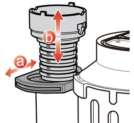
9. To adjust the height of the overflow pipe, slide the lock (a), then set the desired height of the overflow pipe (b). Put the lock back after.
