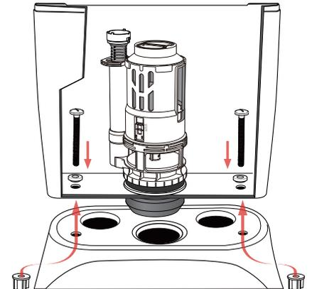
6. Insert the tank to bowl with one pair of plastic or stainless steel bolts through the holes. Insert washers on bolts and screw on the nuts.
