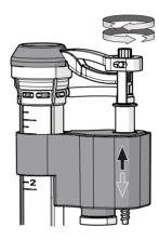
4.Fine and final adjustment can be made by rotating the screw rod clockwise or counterclockwise on the fill valve cup. In order to achieve desired water level;
