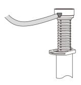
2.Connect the refill tube with refill rest-rictor from fill valve to the overflow pipe of the flush valve;
