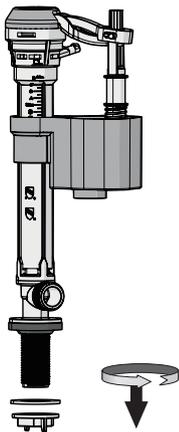
1. Unscrew lock nut and flat washer from fill valve.
