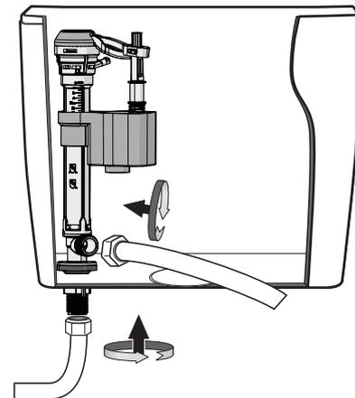
3. Install the water pipe on the fill valve.
