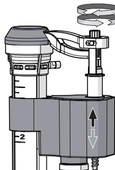
5. Adjust the screw to adjust the water level to the proper line inside the tank.
