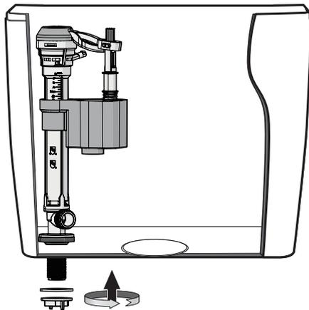
2. Position the fill valve with rubber gasket into the inlet hole of water tank and screw the lock nut with collar tightly. Caution!!! Do not over tighten the nut.
