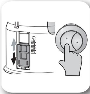
10. Press Full Flush button. Ensure bowl empties sufficiently, and siphon action is activated. If siphon action is not activated, adjust Full flush setting (red) down one notch to 4.5. Press Full Flush button again. Repeat this process until bowl empties and siphon action is activated.
